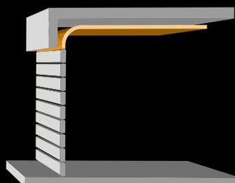
For example, the low-header version is useful in underground and multi-storey car parks.
