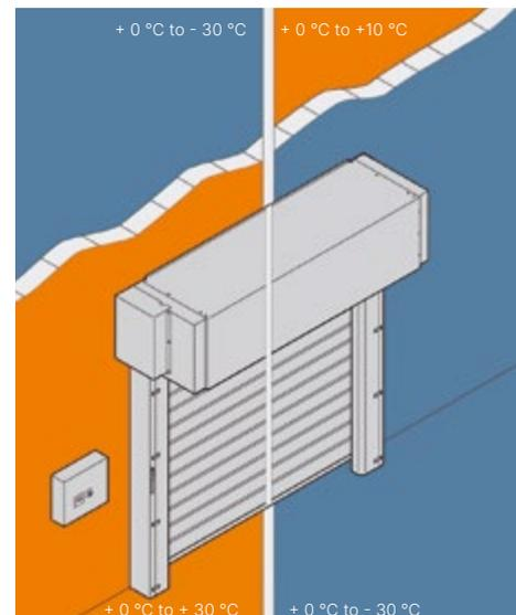
The integrated contact surface heating allows for operating temperatures between plus 30 °C and minus 30 °C.
