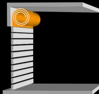
The round spiral is standard and the ideal solution when you have sufficient space above the door.
